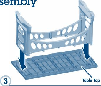
Lay a table top with the bottom side up on a flat surface.Fit the leg assembly into the grooves in the table top.
